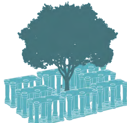
Zuccotti Park in New York applied structural soil under the plaza pavement to create more public space.
